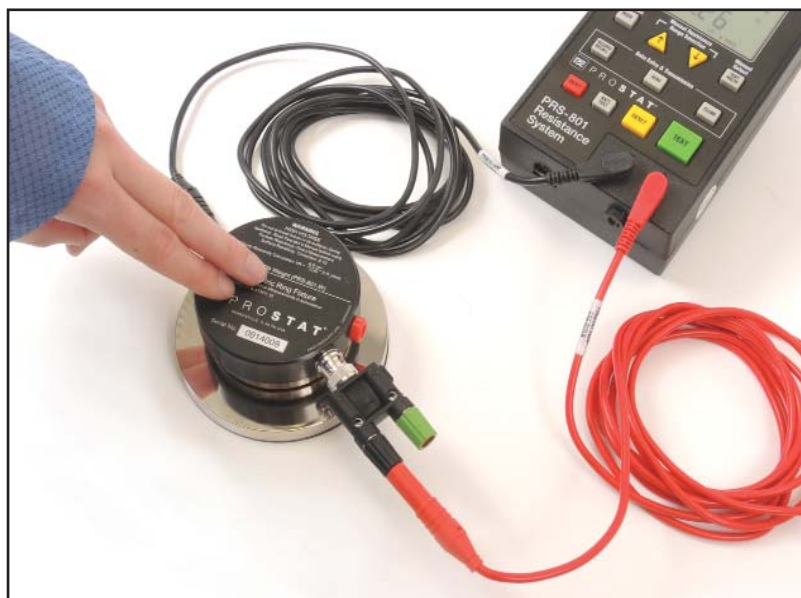
Figure 8: Confirming Electrode Contact to Test Bed
