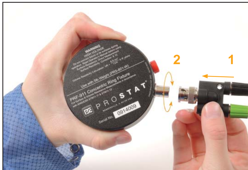
Figure 4: Installing the BNC Adapter
