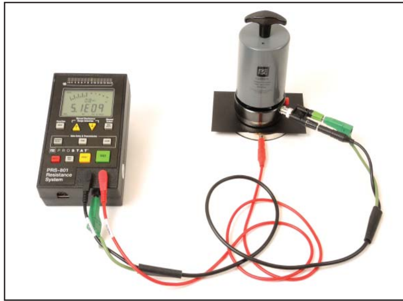
Figure 11: Fixture Preparation (Continued from Fig. 10)
