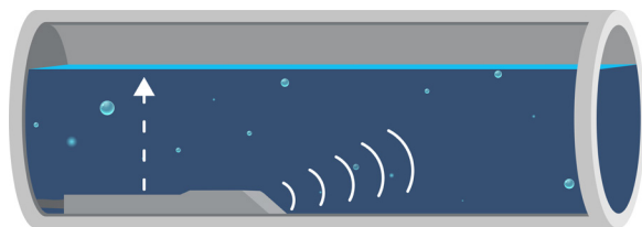
Submerged ultrasonic sensor measures level and velocity
