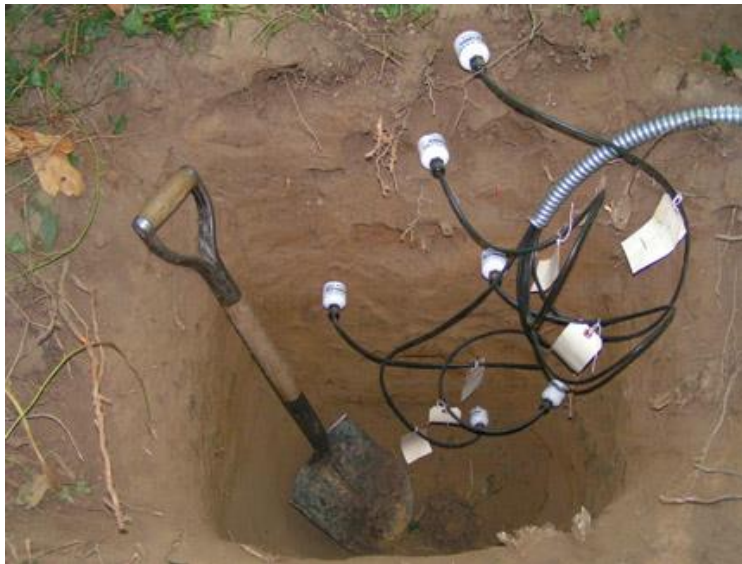
Figure 2.3 Six HydraProbes installed into 6 distinct soil horizons.
