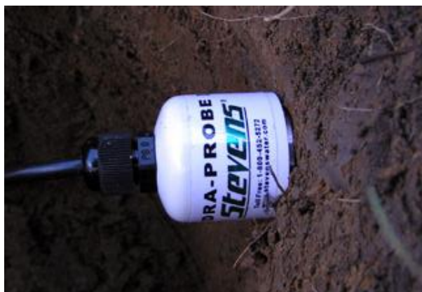
Figure 2.6 HydraProbe Installed in undisturbed soil.
