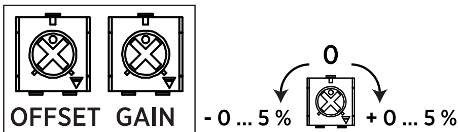
Figure 14 Trimmers for Offset and Gain
