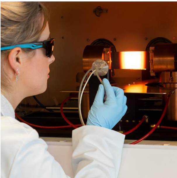
Figure 2 GG01 sensor in a high heat flux test cabinet. Each sensor is tested at its rated measurement range.
