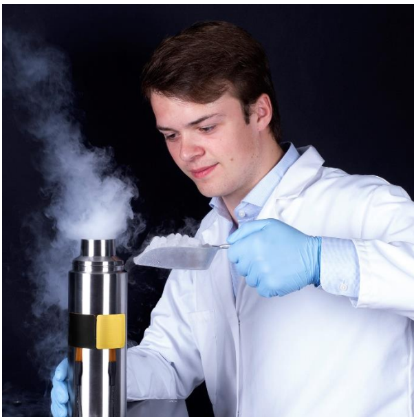
Figure 7 FHF05-50X50 with BLK GLD stickers for measuring insulation losses of a thermos.
