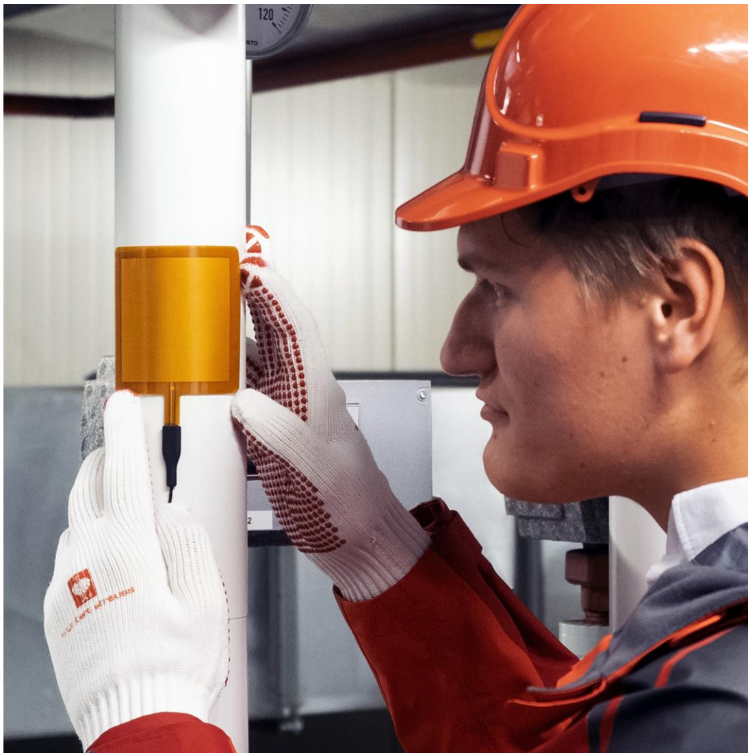
Figure 4.1.1 Example of model FHF05-85X85 foil heat flux sensor being installed for measurement on an industrial pipe. The sensor is mounted on a well-prepared curved surface.
