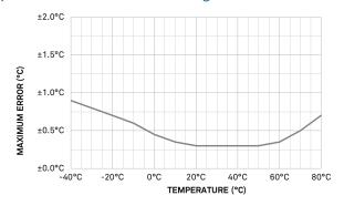
Figure 5 Temperature sensor accuracy
