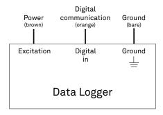
Figure 3 Wiring diagram
