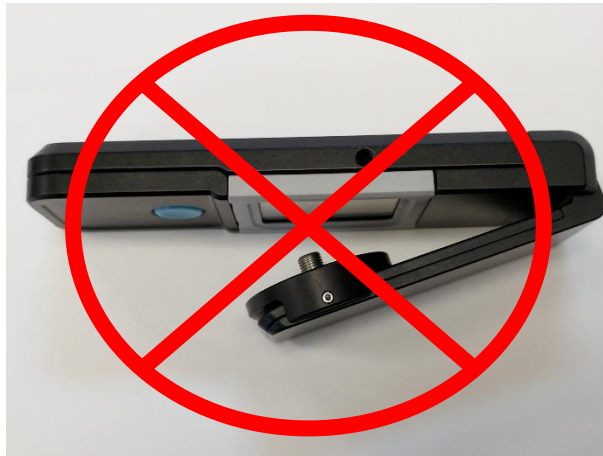
Figure 12. Flipping the PRONTO-Si closed when the FC adaptor is attached will damage the touchscreen
